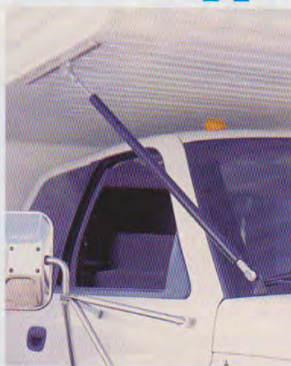
Cabover stabilizers help absorb the bumps while driving on the open road. They act as camper shock absorbers. This new design is a Lance exclusive.
